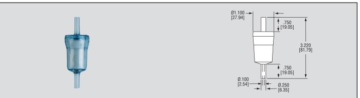
Remove 99.99% of unwanted particles from within your gas flow with the Model F195 Disposable In-Line Filter. Encapsulated microfiber filter elements are able to filter particles as small as 0.1 micron. Filters are completely disposable — simply remove the filter from your line and throw it away when it becomes dirty. The transparent nylon housing makes it simple to determine if the filter needs to be changed.
