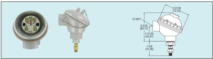
The Model A-709 Temperature Enclosure can be used to mount our Series 651 and 659 transmitters to any of our 1/4 diameter temperature sensors. The screw on enclosure core can be quickly removed and has a chain to prevent it from getting lost. The Model A-709 comes with the necessary adapters and fittings for attaching the temperature sensor.
