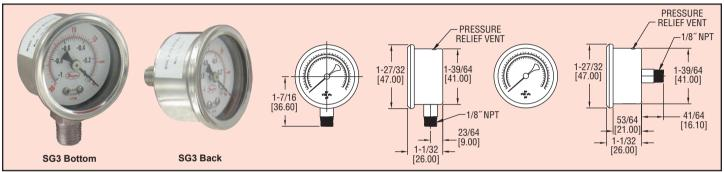
The Series SG3 Gages have dual psi and bar (x100 kPa) scales with ±2.5% full-scale accuracy. The Series SG3 gages are designed with 304 SS housings and 316 SS wetted parts for excellent chemical compatibility. These gages cover a wide variety of ranges from full vacuum to 300 psi. Units can withstand ambient temperatures up to 140°F (60°C). Bottom or back 1/8" NPT connection options available.
