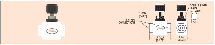
The Model TNV PTFE Needle Valve is designed for laboratory and industrial applications for regulating corrosive gases and liquids for high purity services. Media only come in contact with PTFE and PCTFE. Valve spindles are made of ridged PCTFE to minimize "creeping" normally associated with PTFE. The TNV is designed to be used in pressure or non-critical vacuum applications and can be used as a shut off valve.
