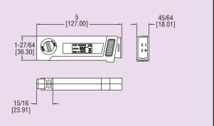
The Series TP2 Thermocouple Thermometers can accurately measure a large temperature range for a wide range of applications including food, safety inspection, lab testing, and HVAC. This hand-held thermometer offers three models that measure the probe temperature, ambient temperature, and relative humidity. Additional features include a data hold function, high/low audible alarm, and auto power off. Device includes a K type probe and battery.
