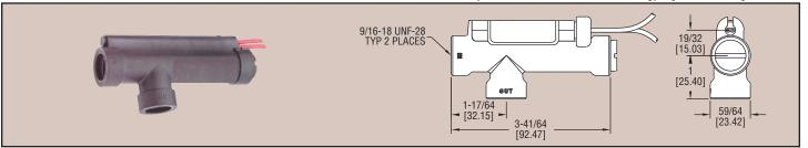
The Series P4 PPS Flow Switch features a molded plastic construction for enhanced performance. Monitor liquids with fixed set points from 0.1 to 1.5 GPM. Choose normally open or normally closed SPST or SPDT hermetically sealed reed switch technology. The industrial switch features PPS R4 housing and piston, 316SS spring, Fluoroelastomer Oring and Epoxy. The inlet and outlet ports are 9/16~-18 UNF-28 thread with optional 1/8″ and 1/4″ NPT or 1/2″ barbed adapters.
