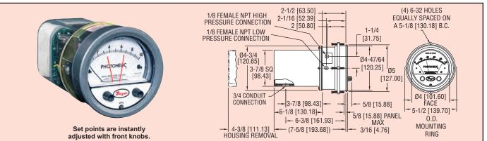
Photohelic<sup>®</sup> Switch/Gages function as versatile, highly repeatable pressure switches combined with a precise pressure gage employing the time-proven Magnehelic® gage design. The Photohelic® gage measures and controls positive, negative or differential pressures of air and compatible gases. Standard models are rated to 25 psig (1.7 bar) with options to 35 (2.4) or 80 (5.5 bar) psig. Single pressure 36000S models measure to 6000 psig (413 bar) with a 9000 psig (620 bar) rating.
