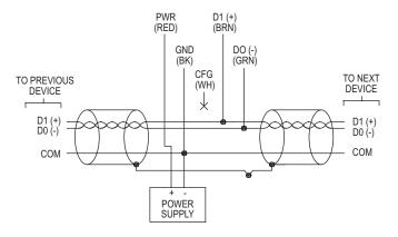
Figure 3: BACnet individual power supply wiring
