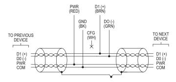
Figure 2: BACnet common power supply wiring
