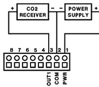
Figure 3: Active output wiring diagram
