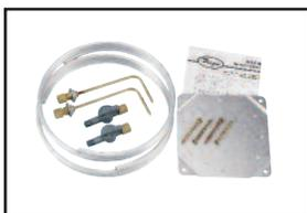
Air Filter accessories furnished are mounting panel with necessary screws, two static pressure taps with integral compression fittings, two five foot lengths of 1/4" aluminum tubing and the two molded plastic vent valve with compression fittings.
