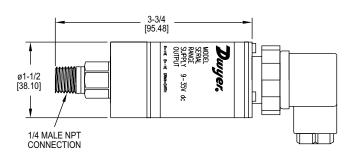
**The Series 672 Low Pressure Transducer** is a perfect solution to any application where a very accurate low pressure transducer is necessary. Using variable capacitance technology, the series 672 is designed to measure pressures as low as 10<sup>°</sup> w.c. up to 400<sup>°</sup> w.c., very low ranges for a single pressure transducer. The 672 also features a 0.25% F.S. accuracy. Use the Series 672 in liquid level, flood warning, waste water, clean room, and open channel flow applications.
