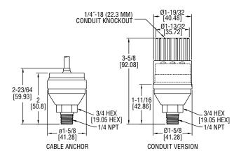
**The low cost Series 673 Pressure Transmitter** is a fixed range transmitter designed for harsh environments and suitable for high shock and vibration applications. Constructed of stainless steel, the Series 673 provides a 4-20 mA output signal with 0.25% accuracy. Use the Series 673 in industrial OEM equipment, hydraulic systems, HVAC equipment, industrial engines and compressor controls.
