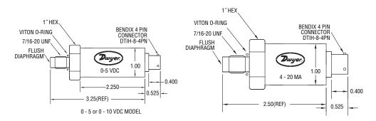
The Series FDT Flush Diaphragm Transmitter is designed for highly cyclical conditions. This unit has a non-oil filled sensor element that provides resistance to temperature fluctuations. Manufactured from a solid piece of steel, the sensing diaphragm can withstand the most abrasive/cyclical applications. Unit performs well in high cyclical environments with the presence of water-hammering or spiking.
