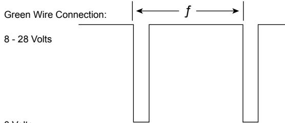
$$GPM = \frac{\text{Freq (Hz)}}{2.0} \quad \text{for SFI-100T-1/2"-A711T}$$
