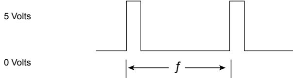
$$GPM = \frac{\text{Freq (Hz)}}{2.0} \quad \text{for SFI-100T-1/2"-A711T}$$
