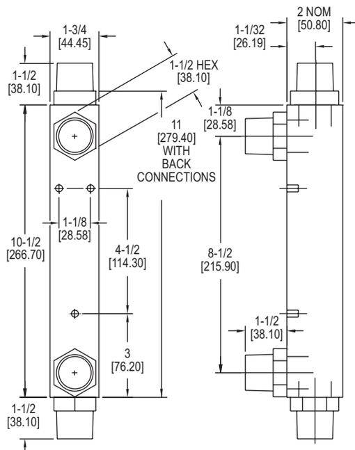
The **Series VFC Visi-Float® Flowmeter** is available in two basic styles, either back or end connected with direct reading scales for air or water. Installation, operation, and maintenance are simple and require only a few common sense precautions to assure long, accurate, trouble-free service.
