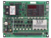
Series DCT dust collector timer controller
