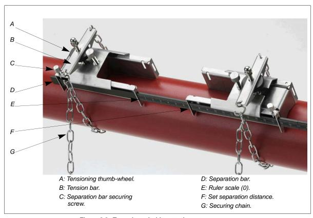
Figure 2.2 Transducer holder attachment
