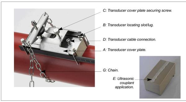
Figure 2.3 Fitting the transducers
