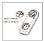
• Insert New 3V lithium battery CR2032 into battery compartment.
