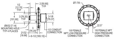
The unique electric switch design in the **Series 1640 Floating Contact Null Switch for High and Low Actuation** is another Dwyer Instruments, LLC innovation. The Dwyer<sup>®</sup> Model 1640 Differential Pressure Switch resembles the high precision large diaphragm Series 1630 switches. However, the Model 1640 is equipped with a single pole, double throw floating contact switch (not snap acting) so it functions as a null switch.
