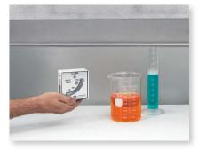
Use a Vaneometer<sup>™</sup> swing vane anemometer to measure velocity of air flow into laboratory fume hoods and at paint spray booths to determine when to change filters. Or wherever needed to meet OSHA standards of ventilation for smoke, dust or fume removal.
