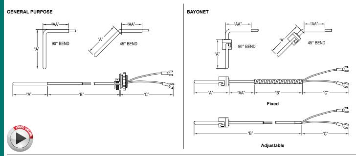
Series 4 & 5 General Purpose and Bayonet Type Thermocouples & RTD's tip temperatures can be as high as 842°F (450°C) for fiberglass insulated wire, and 392°F (200°C) for FEP insulated wire. Models can be specified with lead wires or head assembly construction. For higher temperatures see the Series R & 8 Mineral Insulated Probes.
