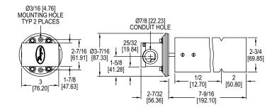
The **Model 530 Air Flow Switch** provides excellent sensitivity and reliability at a very reasonable price. Quality features include a rugged die cast body, stainless steel vane and SPDT snap switch. Unit is field adjustable from 400-1600 FPM. Mounting is fast and simple, with only two screws needed. Vane fits 6 in. or larger ducts.
