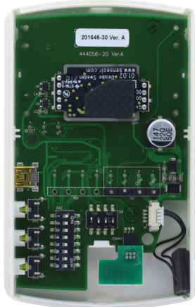
Figure 6: Internal view of transmitter
