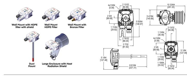
The **Series RHPX Humidity and Temperature Transmitter** offers field selectable voltage and current output for humidity with an active temperature output or a passive temperature sensor connection. Featuring capacitive polymer humidity sensors, models are available in 2% and 3% accuracies.
