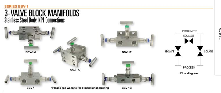
The Series BBV-1 3-Valve Block Manifolds can be used over a broad range of industrial applications including oil refineries, nuclear power stations, petrochemical processing, and more. The Series BBV-1 body is forged from 316 stainless steel bar stock and designed to withstand repeated open and close operations. Suited to control oil, water, toxic fluids, chemicals, air, and steam.
