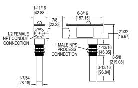
The **Model CLS1 Capacitance Level Switch** provides reliable point level measurement of solids, liquids and slurries in metallic or non-metallic tanks and vessels. It detects the presence or absence of material in contact with the probe by sensing a change in the capacitance.
