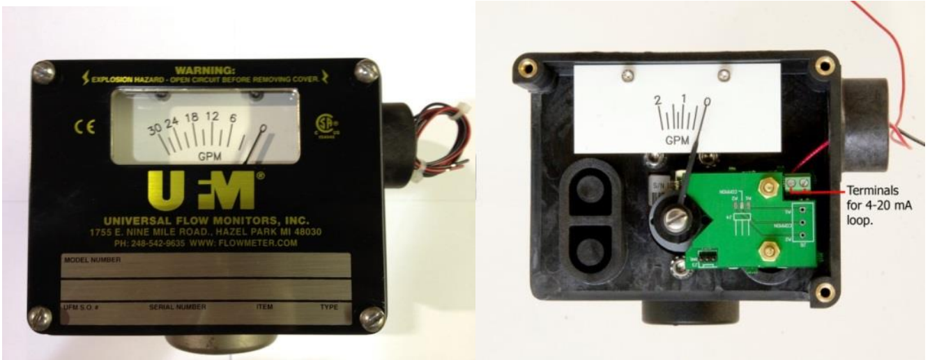
Figure 6: Terminals for 4-20 mA loop
