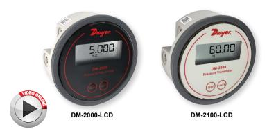
The Dwyer **Series DM-2000 Differential Pressure Transmitters** sense the pressure of air and compatible gases and sends a standard 4-20 mA output signal. The DM-2000 housing is specifically designed to mount in the same diameter cutout as a standard Magnehelic<sup>®</sup> gage. A wide range of models are available factory calibrated to specific ranges.
