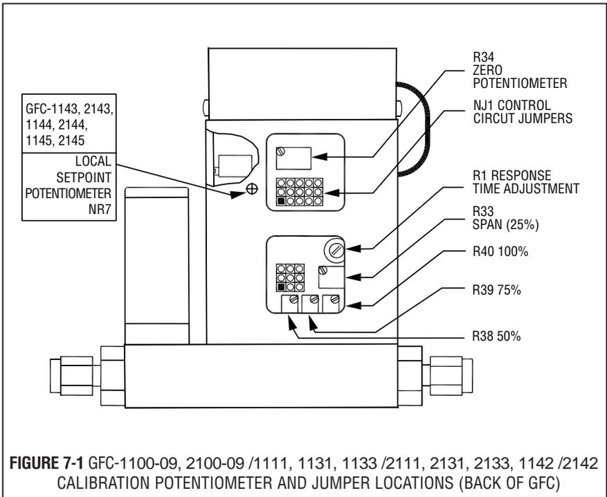
**FIGURE 7-1 GFC-1100-09, 2100-09 /1111, 1131, 1133 /2111, 2131, 2133, 1142 /2142 CALIBRATION POTENTIOMETER AND JUMPER LOCATIONS (BACK OF GFC)**
