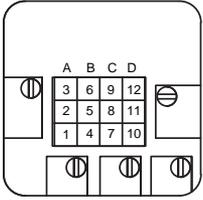
**FIGURE 7-2** GFC-1100-09, 2100-09 /1111, 1131, 1133 /2111, 2131, 2133, 1142 /2142 CALIBRATION POTENTIOMETER AND JUMPERS
