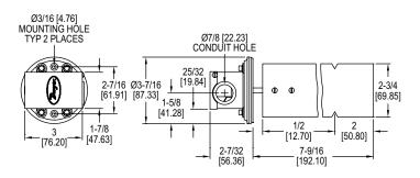
The **Model 530 Air Flow Switch** provides excellent sensitivity and reliability at a very reasonable price. Quality features include rugged die cast zinc body, stainless steel vane, silicone rubber gasket and SPDT snap switch. Unit is easily field adjustable from 400-1600 FPM. Mounting is fast and simple, requiring only two screws. Vane fits 6 in. or larger ducts. UL listed. To order, specify Dwyer Instruments, LLC Model 530 Air Flow Switch.
