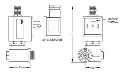
The Series PV three-way normally closed electro-pneumatic solenoid pilot valve effectively regulates supply pressures for the Series SAV Angle Seat Valve. The DIN connector is reversible 180 degrees to keep electrical wiring hassle-free, while the direct mounting banjo connection simplifies valve installation. Select the proper model according to the SAV valve actuator diameter and power requirements.
