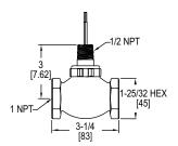
The Series GVS Globe Valve Switch offers accurate flow detection with 1% repeatability and external adjustability over a broad range of flow settings for compatible liquids.
