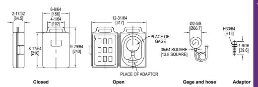
The Series LPTK Gas Pressure Test Kit is ideal for testing LP and natural gas lines and controls. The kit's gage shows if proper pressure is present or if a leak exists. Series LPTK is easier to use than a manometer and includes a sturdy case for added durability and safe handling.
