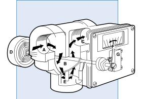
Fluid enters at **A**, passes around the semi-circular vane **B**, exits at outlet **C**. The vane resists the flow because of the spring **D**. The further the vane is pushed the larger the passageway **E** becomes. This minimizes the pressure drop. The vane shaft turns to operate the pointer **F** and remote signal devices such as the switch **G**.
