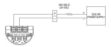
Figure 4-2: Wiring the 3100 pressure transmitter
