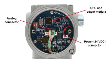
Figure 6-3: Structure of electronics module
