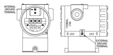
3100 Smart Pressure Transmitter Internal and External Ground Terminal
