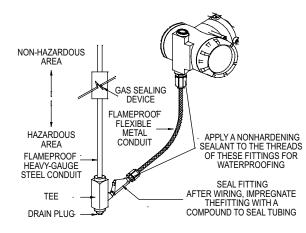
Figure 4-4b: Typical wiring using explosion-proof conduit
