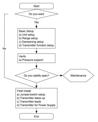
Figure 4-1: Installation flow chart
