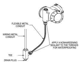
Figure 4-4a: Typical mounting using flexible metal conduit
