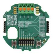
Figure 5: 5 in w.c. pressure board
