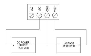
Figure 2: DC wiring
