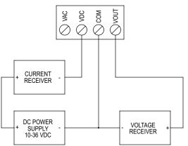
Figure 4: Simultaneous current and voltage output wiring
