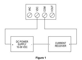
The maximum receiver load resistance (RL) for a given power supply voltage (Vps) is defined by the formula:
