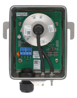
Figure 5: 5 in w.c. pressure board
