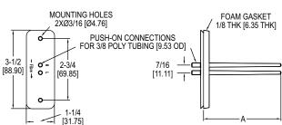
The **Series PAFS-1000 Averaging Flow Sensors** are ideal for sensing velocity pressure in the inlet section of variable air volume terminal units and fan terminal units.
