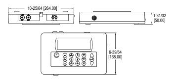
The Series PUB & PUF Portable Ultrasonic Flowmeter Kits utilize the transit-time difference for measuring flow rates in pipes non-invasively. Units offer flow rate local display with analog and pulsed outputs. The Series PUF offers the same features plus data logging capability.
