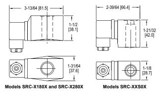
The **Series SRC Solenoid Replacement Coils** electrically operate the SSV and SBSV solenoid valves. When the solenoid coil receives an electrical input signal it acts upon the valve, changing its state. These coils are field replaceable with their compatible solenoid valves and come in a wide range of voltages.
