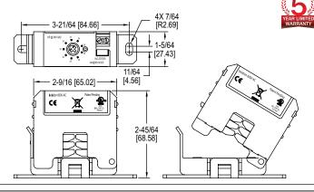
The Series SSCS Sure-Set Current Switches provide a unique approach to calibration and installing current sensors in a low cost, fast, and accurate design. Selecting the set point has never been easier, with each model having 9 pre-configured adjustable HP set points. This feature eliminates the need to work within a live enclosure, reducing the risk of arc flash on installation
