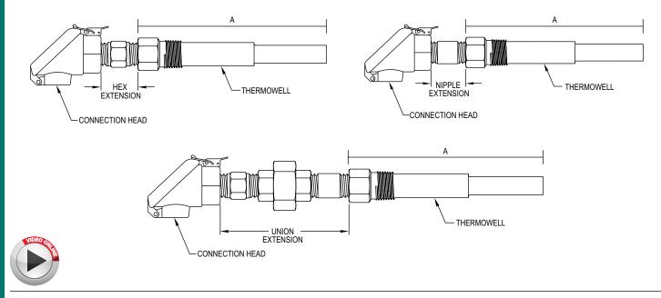
Series T Temperature Sensor Assemblies with Thermowells are available in a variety of head styles and thermowell materials. All elements are spring loaded to ensure positive contact in the thermowell. Thermowells are non-lagging. The sensor sheath material is constructed of 316 SS regardless of the well material specified.
