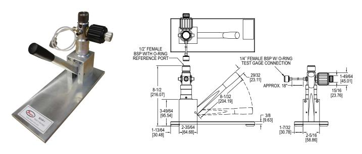
The Series BCHP Low Pressure Hand Pump is able to generate pressure and vacuum for adjusting or calibrating pressure gauges, transmitters, or switches. The pump is hand operated and has a pneumatic pressure range of -28 in Hg to 870 psi (-0.95 bar to 60 bar). Dual pressure ports allow two instruments to be connected to the pump without additional fittings. The Series BCHP can be used in laboratories and production areas. The fine adjustment valve on this pump ensures precise measurements
