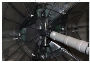
When using the short pole or with the SAH adapter base kit for canvas hoods, the stationary pole adapter should be used to keep the hood pole from pivoting. Place the stationary pole adapter onto the SAH and attach using the screws and wing nuts provided (below). Once secure to the SAH, insert the short pole and secure in place using the locking pin.
