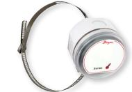
The Series TE-SNW Weather Resistant Surface Temperature Sensor nonintrusively measures the process temperature in hot and cold water loops in buildings. In order to work with most common building controllers, the output of the sensor can be chosen from 6 different RTD and Thermistor curves
