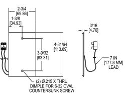
The Series TE-WSS Stainless Steel Wall Plate Temperature Sensor measures the ambient air temperature in classrooms and industrial environments.
