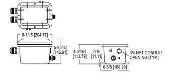
The Series TR-7 Safe-T-Ground provides continuous monitoring of a truck's ground connection throughout loading operations. The TR-7 instantly stops loading operations if a tank truck loses its ground. To safeguard loading operations, the Safe-T-Ground circuit can be wired into your pump control, and to an audible alarm or signal light.
