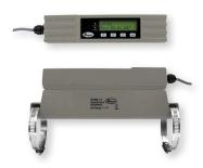
The Series UFM2 Compact Ultrasonic Flowmeters are economical, clamp-on, ultrasonic flowmeters. The UFM2 implements the transit-time difference to measure flow rates in pipes and can measure velocity and flow in pipes with outside diameters ranging from 3/4 to 7" (25 to 180 mm). This model comes with a volume pulse and 4-20 mA flow rate output.
