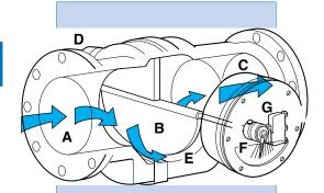
Fluid enters at **A**, passes around the semi-circular vane **B**, exits at outlet **C**. The vane resists the flow because of the spring **D**. The further the vane is pushed the larger the passageway **E** becomes. This minimizes pressure drop. The vane shaft turns to operate the pointer **F** and remote signal devices such as the switch **G**.
